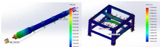
Fig. 2. Strength simulation of spinner machine's main parts
