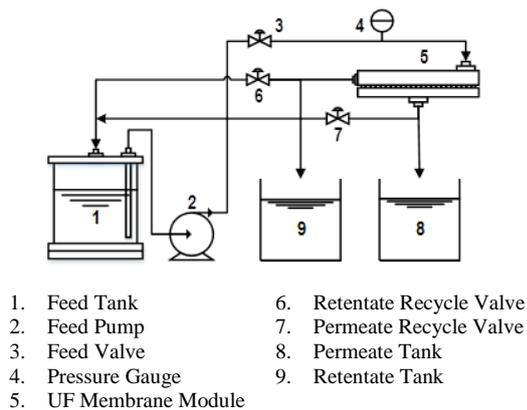
Fig. 2 Schematic of the ultrafiltration cell
