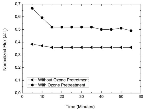
**Fig. 5** Effect of ozonation pre-treatment on membrane normalized fluxes as a function of time for ultrafiltration of produced water (membrane: PES 1, TMP = 1 bar)
