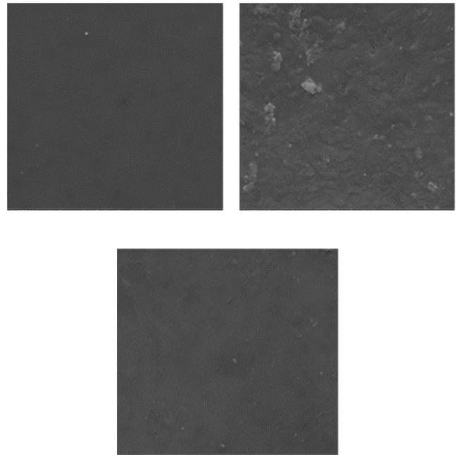
**Fig. 6** SEM result of PES membranes (magnification of 20,000×): (a) clean membrane (before filtration), (b) membrane after filtration without ozone pre-treatment, and (c) membrane after filtration with ozone pre-treatment. (membrane PES 1, TMP = 1 bar)
