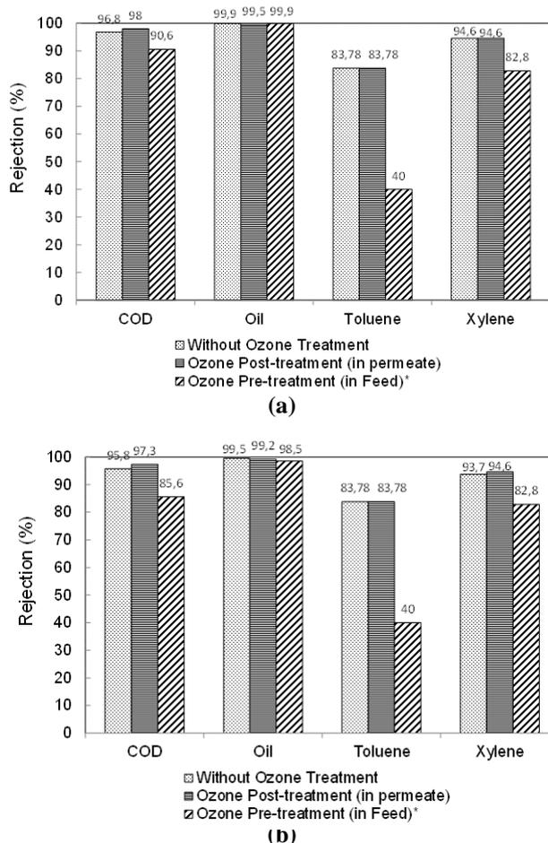
**Fig. 7** Rejection of COD, oil, toluene, and xylene under various conditions (TMP = 1 bar): (a) PES 1 and (b) PES 2 \* (Cf Toluene = C Toluene after feed ozonation = 0.10 mg/L).
