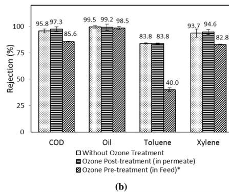
**Fig. 7** Rejection of COD, oil, toluene, and xylene under various conditions (TMP = 1 bar): (a) PES 1 and (b) PES 2 \* (C, Toluene = C Toluene after feed ozonation = 0.10 mg/L).
