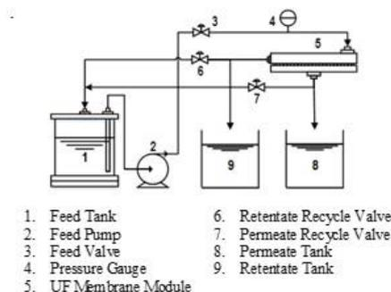
**Fig. 2** Schematic of the ultrafiltration cell
