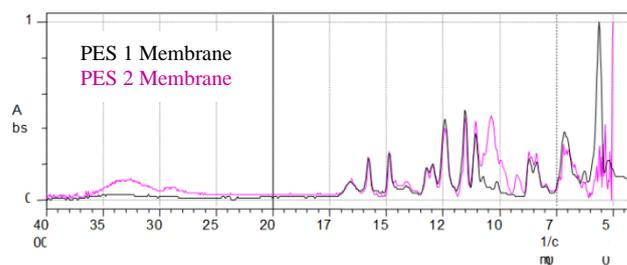
Fig. 1 FTIR results of PES 1 and PES 2 membranes
