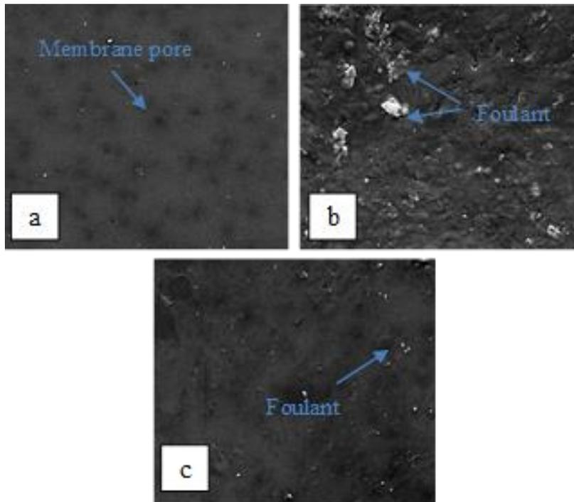
**Fig. 6** SEM result of PES membranes (magnification of 20,000×): (a) clean membrane (before filtration), (b) membrane after filtration without ozone pre-treatment, and (c) membrane after filtration with ozone pre-treatment. (membrane PES 1, TMP = 1 bar)
