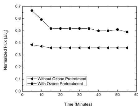
Fig. 5 Effect of ozonation pre-treatment on membrane normalized fluxes as a function of time for ultrafiltration of produced water (membrane: PES 1, TMP = 1 bar)
