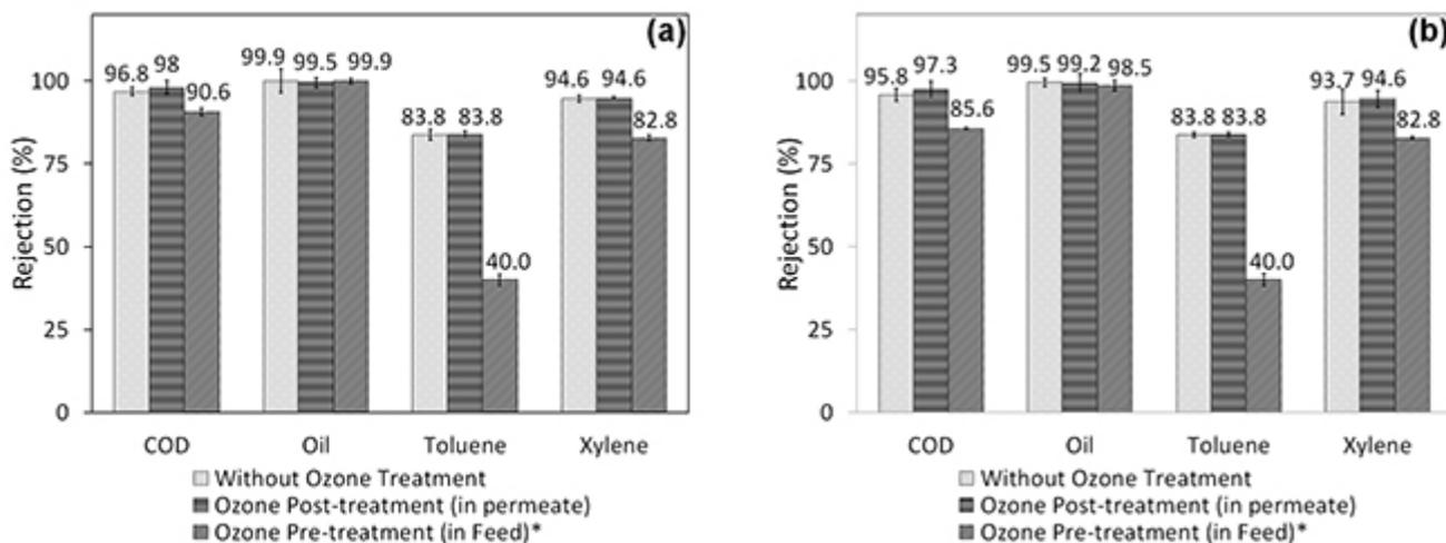
**Fig. 7** Rejection of COD, oil, toluene, and xylene under various conditions (TMP = 1 bar): (a) PES 1 and (b) PES 2
