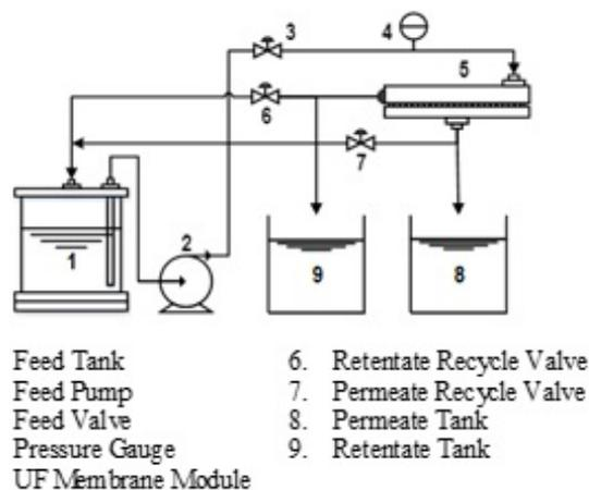
Fig. 2 Schematic of the ultrafiltration cell
