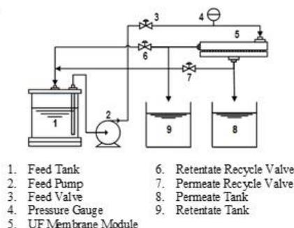
Fig. 2 Schematic of the ultrafiltration cell
