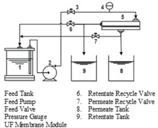
Fig. 2 Schematic of the ultrafiltration cell
