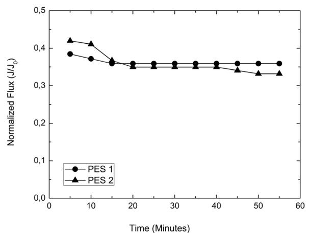
**Fig. 3** Performance of membrane normalized fluxes as a function of time in treatment of produced water by using membranes with different pore sizes (TMP = 1 bar)
