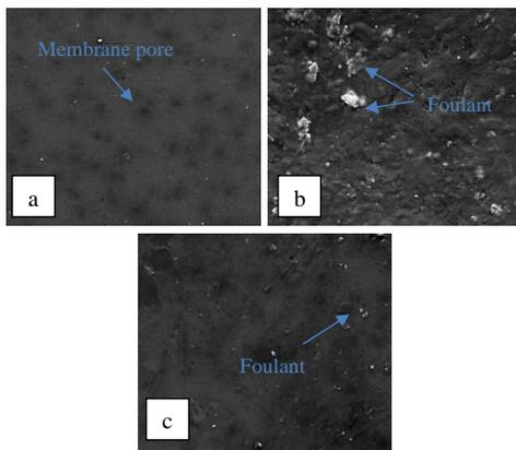
**Fig. 6** SEM result of PES membranes (magnification of 20,000 $\times$ ): (a) clean membrane (before filtration), (b) membrane after filtration without ozone pre-treatment, and (c) membrane after filtration with ozone pre-treatment. (membrane PES 1, TMP = 1 bar)
