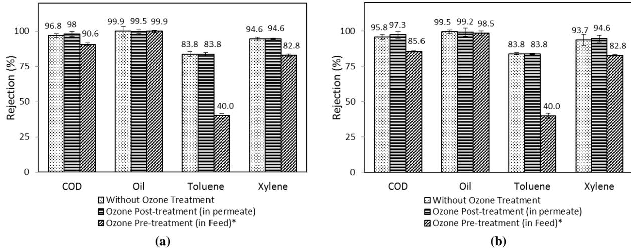
**Fig. 7** Rejection of COD, oil, toluene, and xylene under various conditions (TMP = 1 bar): (a) PES 1 and (b) PES 2 \* ( $C_f$  Toluene =  $C$  Toluene after feed ozonation = 0.10 mg/L)
