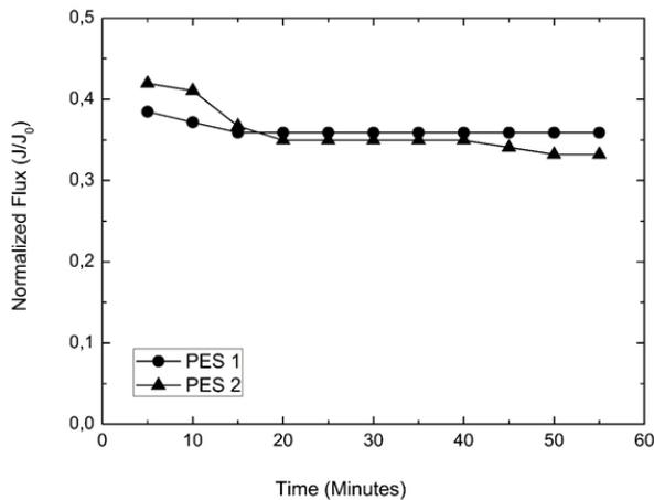
**Fig. 3** Performance of membrane normalized fluxes as a function of time in treatment of produced water by using membranes with different pore sizes (TMP = 1 bar)
