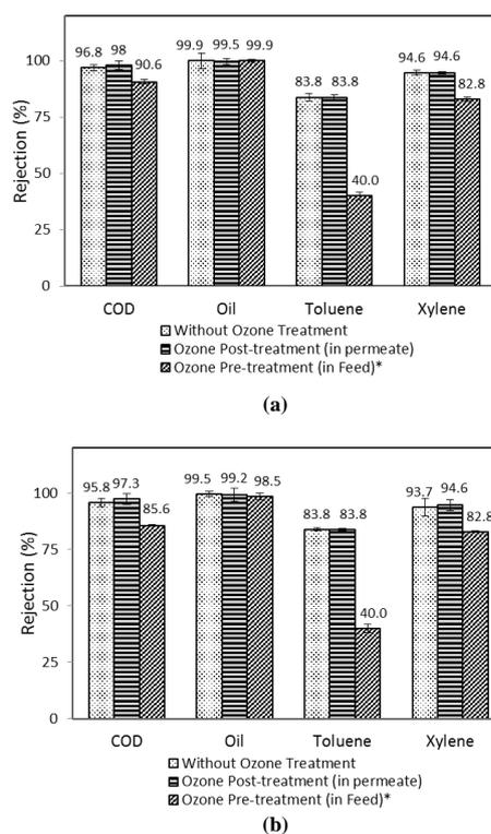
Fig. 7 Rejection of COD, oil, toluene, and xylene under various conditions (TMP = 1 bar): (a) PES 1 and (b) PES 2 \* (C<sub>7</sub>Toluene = C<sub>8</sub>Toluene after feed ozonation = 0.10 mg/L).
