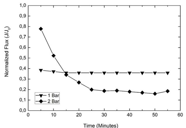
**Fig. 4** Behavior of membrane normalized fluxes as a function of time in treatment of produced water under different trans membrane pressure levels (membrane : PES 1)
