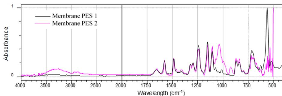
Fig. 1 FTIR results of PES 1 and PES 2 membranes
