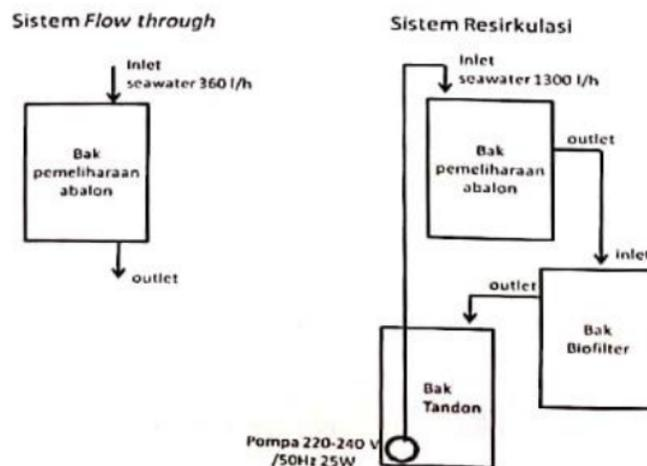
Gambar 1. Skema sistem flow through dan resirkulasi
