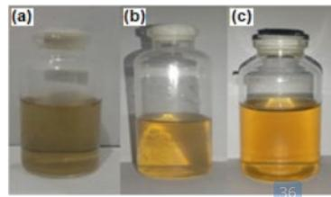
Fig 2. Colloidal AgNPs synthesized by pulsed laser ablation technique in liquid medium (a) PEG, (b) PVP, and (c) Chitosan
