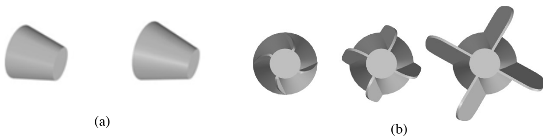
Figure 2. Propeller cap model 15° and 20° (a) and PBCF model (b)
