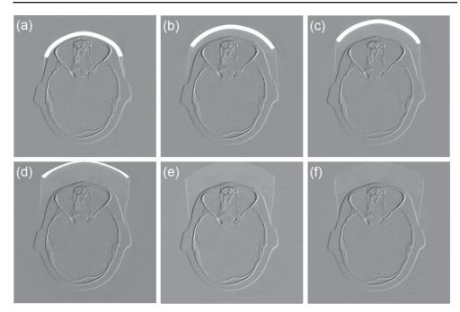
**Figure 11.** Subtraction images between images with the SR-Pb 5% wt eye shield and images without it for various distances; (a) 0, (b) 1, (c) 2, (d) 3, (e) 4, and (f) 5 cm.
