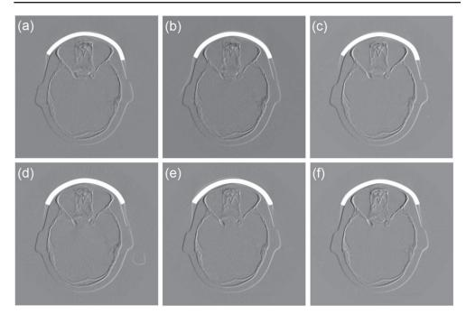
**Figure 8.** Result of subtraction images with and without the SR-Pb eye for various Pb percentages; (a) 0, (b) 1, (c) 2, (d) 3, (e) 4, and (f) 5% wt. The SR-Pb eye shields are on the head.
