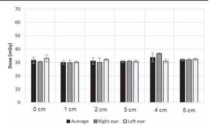
Figure 9. Surface doses at the eyes using the SR-Pb 5% wt eye shield for distances from 0 to 5 cm.
