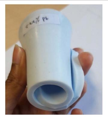
Figure 12. SR-Pb 5% wt eye shield elasticity.
