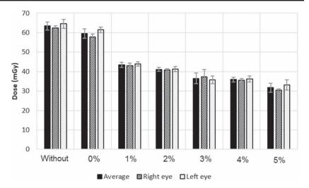
**Figure 6.** Surface doses of eye with and without the SR-Pb eye shield with various Pb percentages from 0 to 5% wt. The standard deviations are shown by bars.
