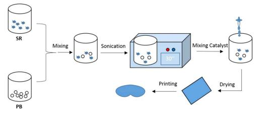
Figure 1. Synthesis of the SR-Pb eye shield.
