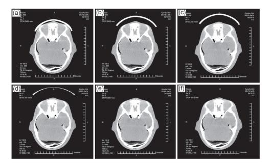
**Figure 10.** Image of head phantom for various distances for the SR-Pb 5% wt eye shield; (a) 0, (b) 1, (c) 2, (d) 3, (e) 4, and (f) 5 cm.
