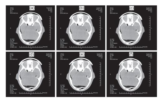
**Figure 7.** Images of head phantom for various Pb percentages with the SR-Pb eye shield. (a) 0 (b) 1 (c) 2 (d) 3 (e) 4 and (f) 5% wt. The SR-Pb eye shields are on the head.
