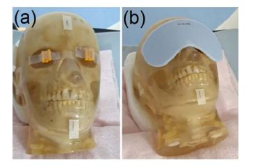
**Figure 2.** (a) PLDs were placed above the surface of the eye on the head phantom, and (b) the eye shield was placed above the head phantom. The distance between the eye shield and the head phantom was varied from 0 cm to 5 cm.
