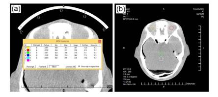
**Figure 3.** (a) Positions of the ROIs to calculate HU of the SR-Pb eye shield and its homogeneity. The size of the ROIs was 6 pixels or about  $1.3 \text{ mm}^2$ . (b) Positions of the ROIs to characterise the amount of artifact by determining HU values in the eye area and the center of the head. The size of the ROIs was 460 pixels or around 100 mm<sup>2</sup>.
