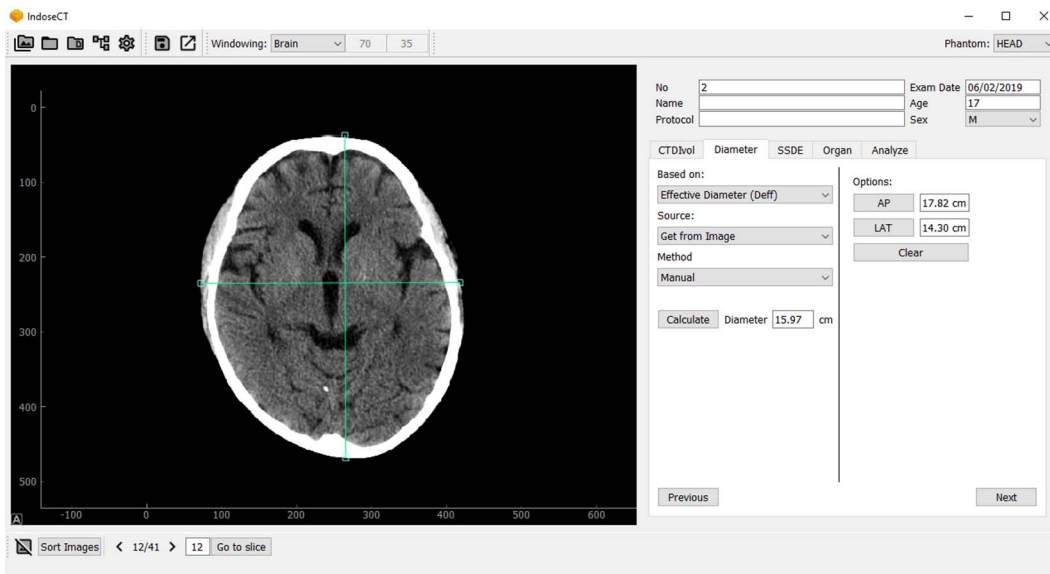
Figure 1. IndoseCT 20b screen display to measure AP dimension and LAT dimension manually.
