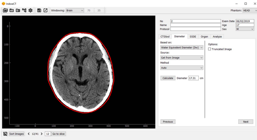
Figure 3. IndoseCT 20b screen display to automatically calculate D_w from patient's image.
