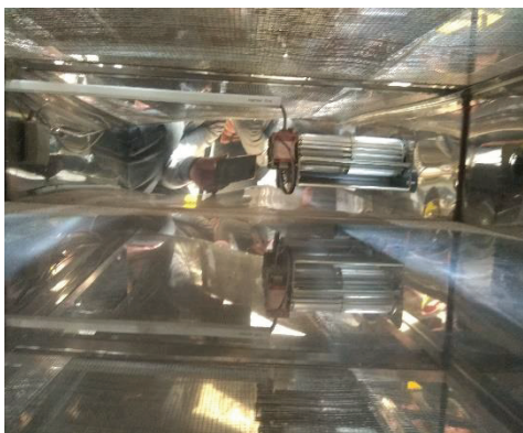
FIGURE 3. View of blower at the bottom of the dryer
