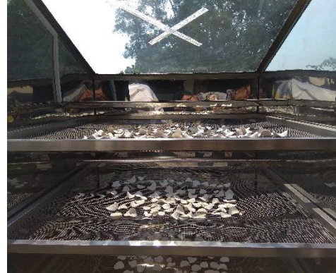
FIGURE 2. Drying trays and inside part of solar dryer
