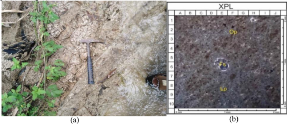
Fig. 5. (a) Claystone unit at STA 11 (b) Petrographic appearance (opaque minerals (Op), clay minerals (Lp), foraminifera fossils (Fs)).
