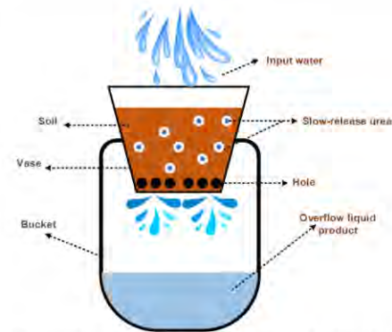
Figure 1. Schematic illustration of the apparatus for slow-release urea performance test.
