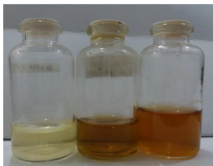
Fig. 8: Colloidal nanoparticles of (a) zinc oxide, (b) iron oxide nanoparticles, and (c) mixture of Zn-Fe.
