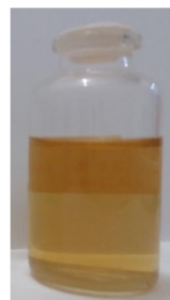
Fig. 6: Colloidal iron oxide nanoparticles produced in PVP medium.
