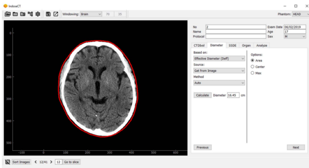
Figure 2. IndoseCT 20b screen display to automatically calculate D_{eff} based on patient image area.
