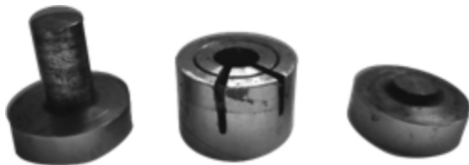
Fig. 4. Tool for Ag 2 S pellet preparation.
