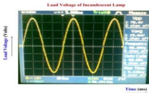
Figure-19. AC load voltage waveform of closed loop seven Level FCMLI system with incandescent lamp load
