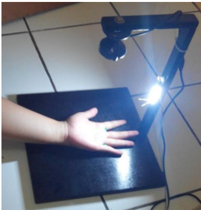
Fig. 4. Hardware of palmprint identification system
