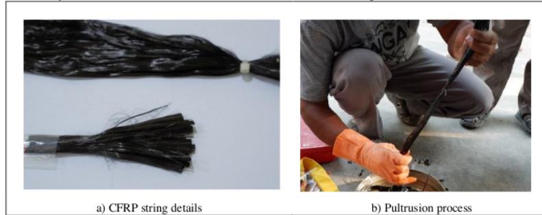
Fig 4. CFRP String Details and Pultrusion
