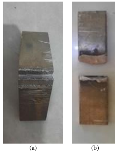
Figure. 10. (a) FSW Specimens After Being Given Bending Test. (b) TIG Specimens After Being Given Bending Test
