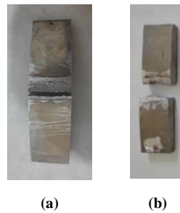
Figure 8. (a) FSW Specimen After Being Given Bending Test. (b) TIG Specimen After Being Given Bending Test.
