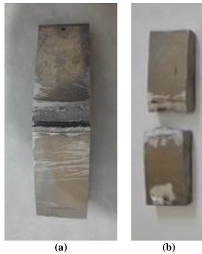
Figure 8. (a) FSW Specimen After Being Given Bending Test. (b) TIG Specimen After Being Given Bending Test.
