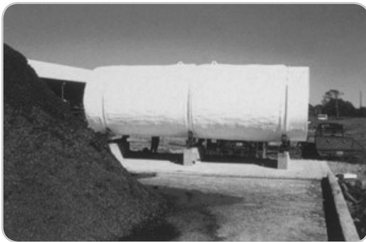
Gambar 12. Sistem In-Vessel Sumber : Mark & Britt, 2009
