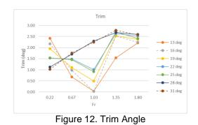
The ship's bow angle engineering could improve the ship's trim condition at a certain speed. At Fr 0.22, there was a decrease in the trim angle of the ship along with the change in the angle of the bow (hull entrance), while at Fr 0.67, there was an increase in the trim angle of the ship along with the change in the angle of the bow of the ship. There was a change in the trim value of the ship due to the difference in the centre of gravity of each ship model with a different bow angle.
