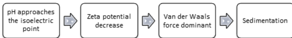
Figure 6. Stages of sedimentation due to the influence of pH
