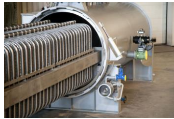
Figure 3.9 Various industrial size pf leaf filter medium
