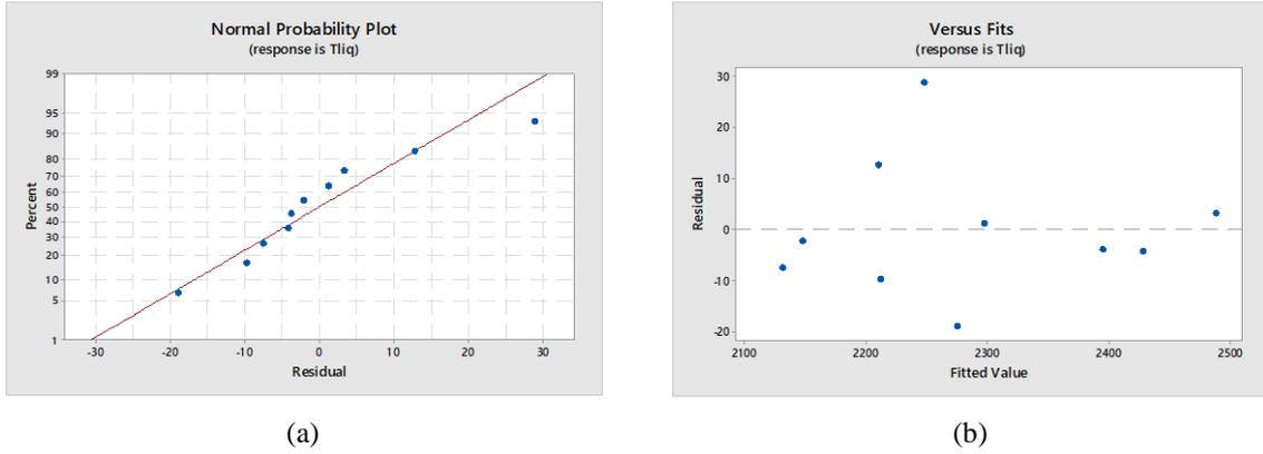
**Fig. 3.** Adequacy checking for special cubic model of geopolymer liquidus temperature: (a) normal probability plot and (b) residual versus fitted value
