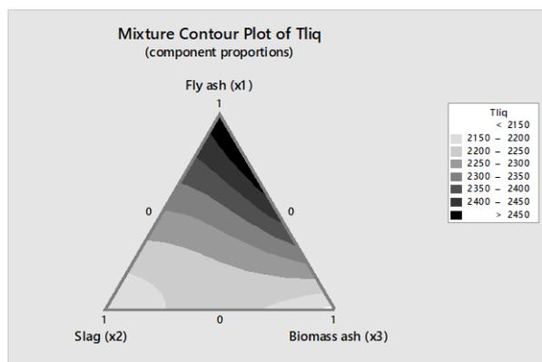
**Fig. 5.** Contour plot of geopolymer liquidus temperature
