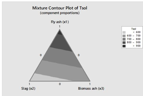
**Fig. 4.** Contour plot of geopolymer solidus temperature
