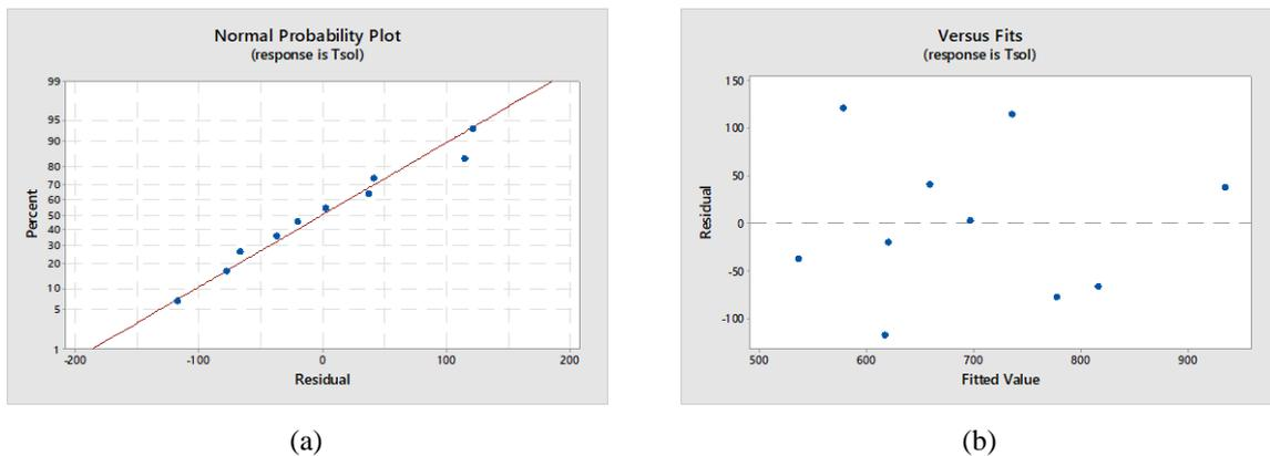
**Fig. 2.** Adequacy checking for linear model of geopolymer solidus temperature: (a) normal probability plot and (b) residual versus fitted value
