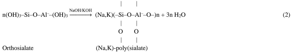
Three-dimensional structure of geopolymer products are amorphous to semi-crystalline and can be poly(sialate)/(-Si-O-Al-O-) for Si:Al = 1:1, poly(sialate-siloxo)/(-Si-O-Al-O-Si-O-) for Si:Al = 2:1, or poly(sialate-disiloxo)/(-Si-O-Al-O-Si-O-Si-O-) for Si:Al = 3:1 [5].
