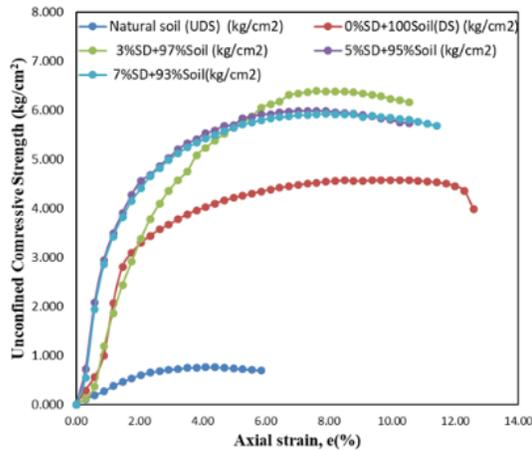
Fig. 2. UCS for different soil-sawdust mixtures.
