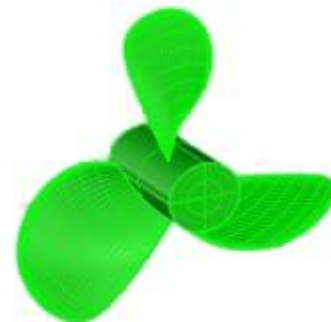
Figure 8. Model B-Series Propeller Type B3-50 on Old Fishing Vessel
