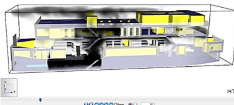
Figure 9. The Result of Fire Simulation Process
