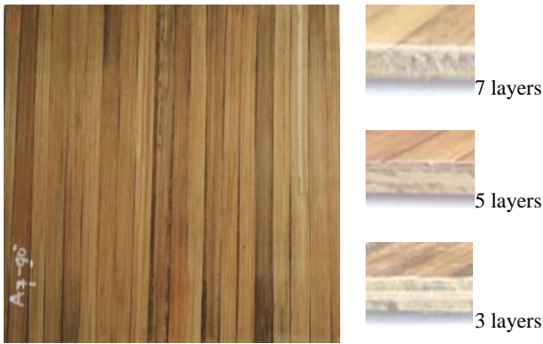
Fig. 7. Bamboo composite board in the crossing degrees direction of 0°/90°
