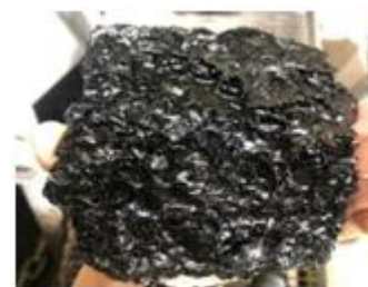
Figure 2: Bottom Ash/Clinker from Boiler
