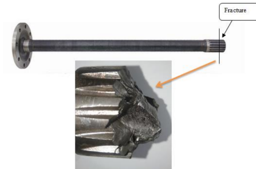
Figure 1: The Broken of the Axle Shaft whos Connected with a Differential Gear
