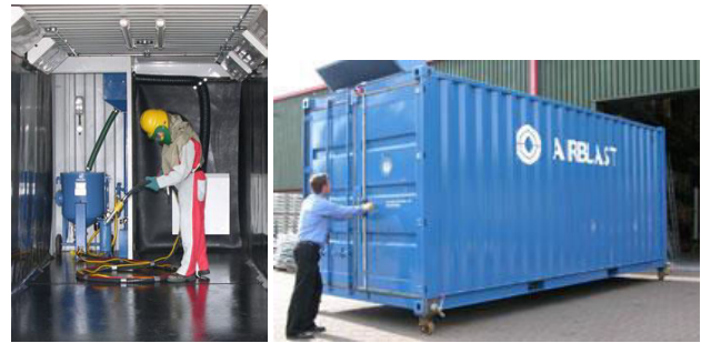
Figure-4. The containerized blast room.
