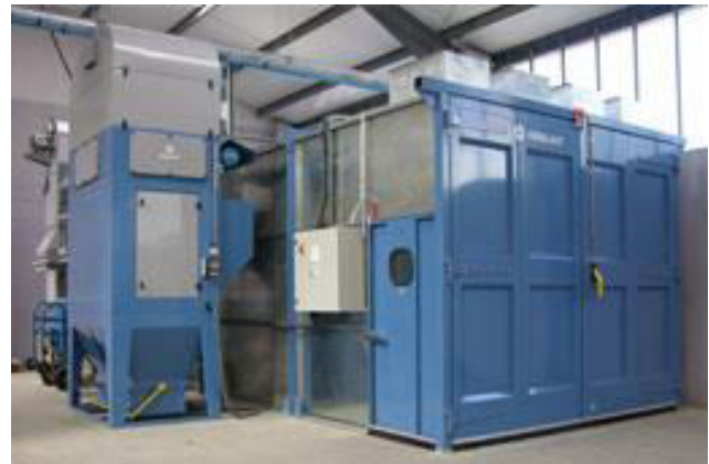
Figure-5. The modular blast room.
