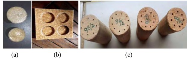
Figure 1. (a) The samples of water hyacinth composite; (b) the Architectural material made of water hyacinth composite; (c) the samples of porous ceramics
