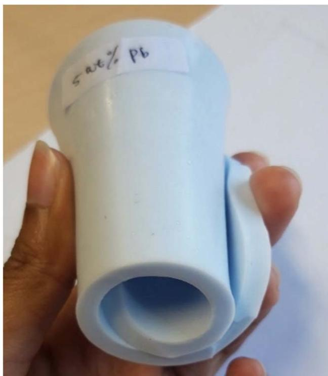
**Figure 12.** SR-Pb 5% wt eye shield elasticity.
