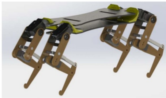
Fig. 1. 3D design of the cat-like robot.
