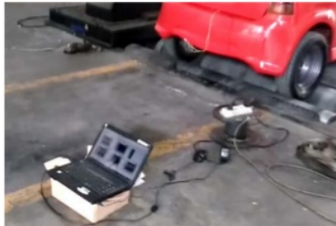
Fig. 13. SOC testing using coulomb counting method
