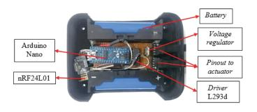
Fig. 6. The prototype of receiver hardware system on the soft glove (controller box)
