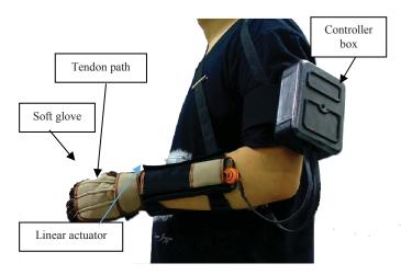
Fig. 7. The prototype of a final wearable soft robotic glove
