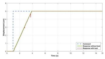
Fig. 8. Step response of soft exoskeleton glove
