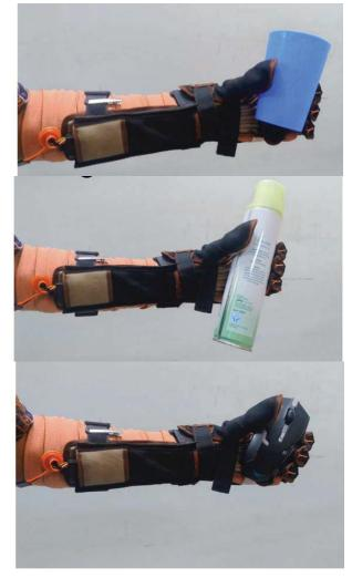
Fig. 9. Performance of the proposed wearable soft robotic glove for assisting various object grasping tests
