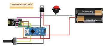
Fig. 3. Proposed transmitter hardware system
