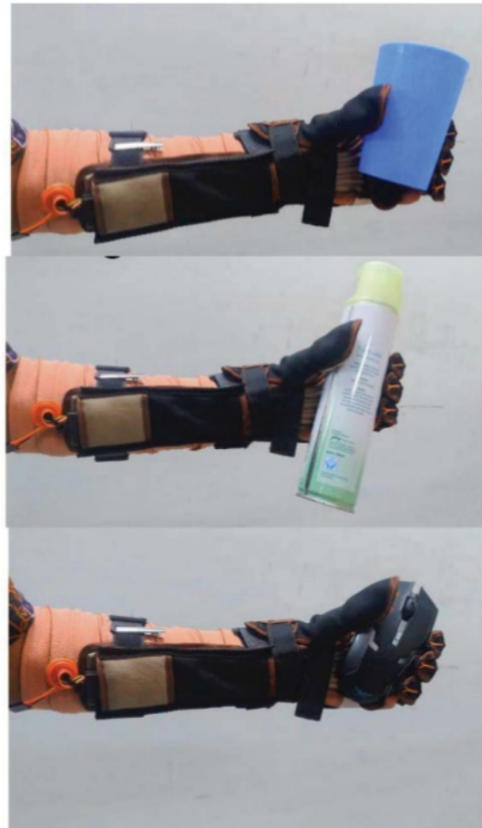
Fig. 9. Performance of the proposed wearable soft robotic glove for assisting various object grasping tests
