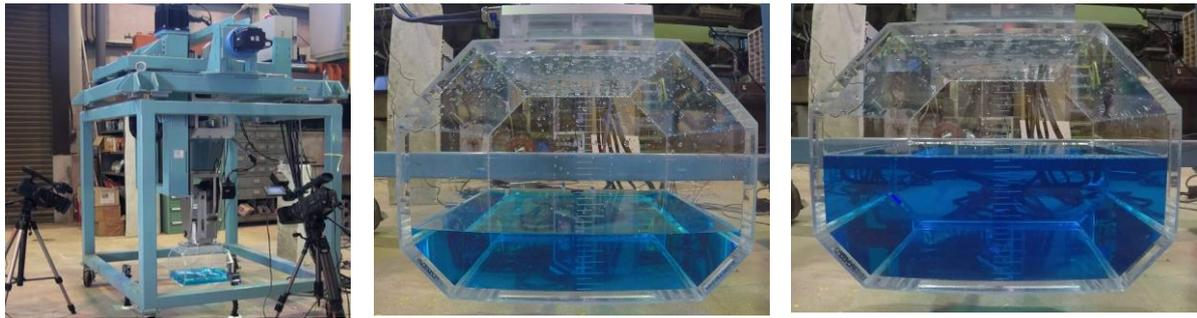
**Fig. 1** Experimental condition of sloshing filling ratio 25% (a), condition of water depth with filling ratio 25% (b), and 50% (c).
