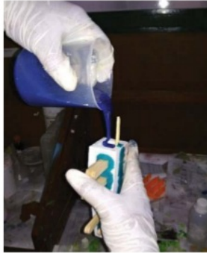
Fig. 5. Pouring the silicone mix to the mold
