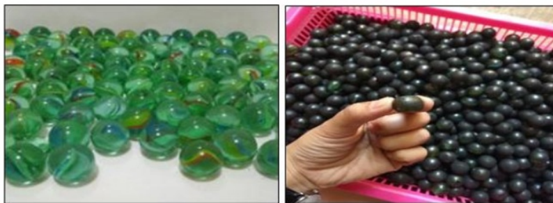
Figure.4 Clean marbles before running (left) and black thickened marbles after running (right)
