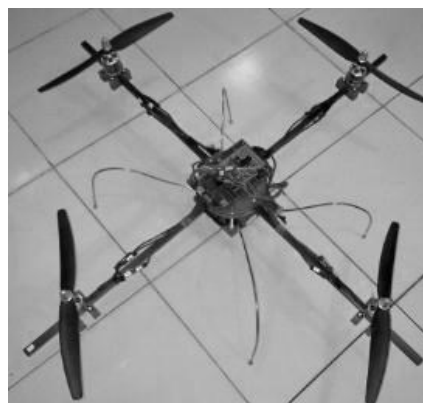
Fig. 1. Quadrotor prototype equipped with gripper at Control Systems and Robotics Lab., Diponegoro University.
