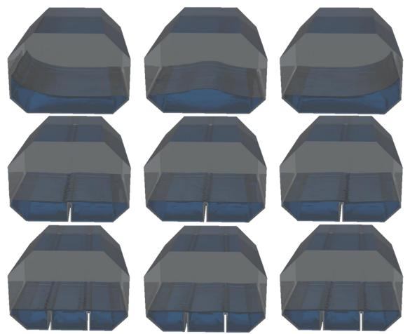
Fig. 9. Comparison of free surface deformation inside tank without and with baffles
