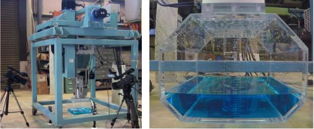
Fig. 1. Sloshing experiment conditions with forced oscillation machine [13]
