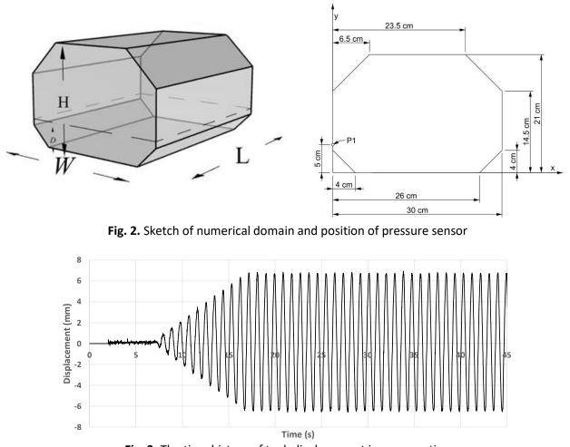
Fig. 3. The time history of tank displacement in sway motion
