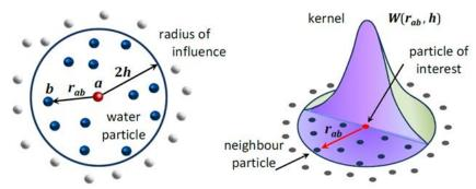
Fig. 4. Radius of the smoothing length and kernel function in SPH [25]
