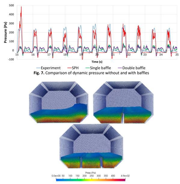
**Fig. 8.** Snapshot of dynamic pressure for sloshing without and with baffles with t = 15.20 s
