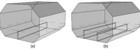
**Fig. 5.** Sketch of the prismatic tank with a (a) single-vertical baffle, and (b) double-vertical baffle
