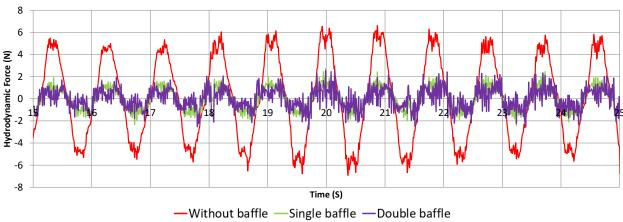
Fig. 10. The hydrodynamic force with and without baffles
