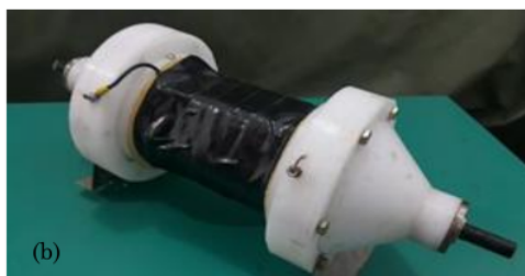
Figure 2. Integrated ozone generator with seven DBD reactors (a) Design (b) Realization
