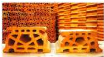
Gambar 1. Penampang segmental keraton (Hazairin et al., 2013)
