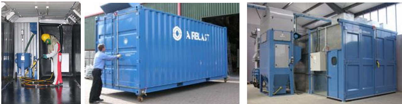
(a) (b) Fig. 1. (a) The containerized blastroom; (b) The modular blastroom
