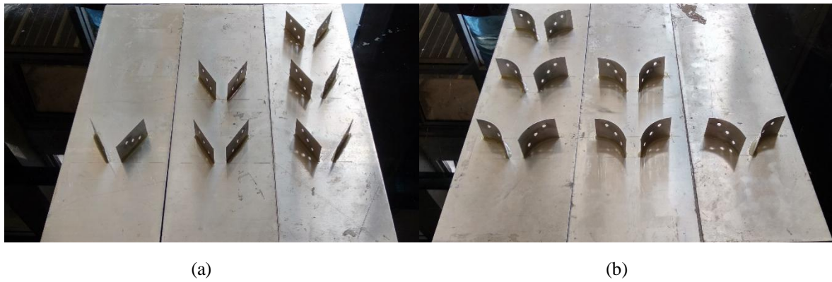
Gambar 3: Spesimen uji: (a) rectangular winglet pair vortex generators(RWP VGs) dan (b) concave rectangular winglet pair vortex generators(CRWP VGs)
