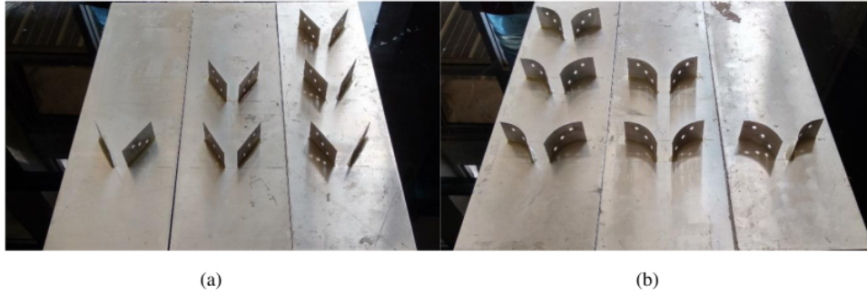
Gambar 3: Spesimen uji: (a) rectangular winglet pair vortex generators(RWP VGs) dan (b) concave rectangular winglet pair vortex generators(CRWP VGs)
