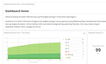
Figure 6 shows the results of the Home dashboard testing which shows the system can receive logs from all network devices and process the log into information according to the type of visualization that has been configured. Through the Home dashboard information about the units that send the
