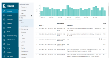
Figure 4 shows the log of network devices successfully received by the server and can represent identification of parts of the message from the log received. The IP address of the device that sent the log can be translated into a hostname and successfully tagged unit based on the hostname. Special
