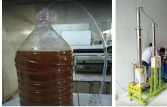
FIGURE 7. Procedure IV: Fermentation process for 6 days and Distillation at Temp. 75°C - 85°C
