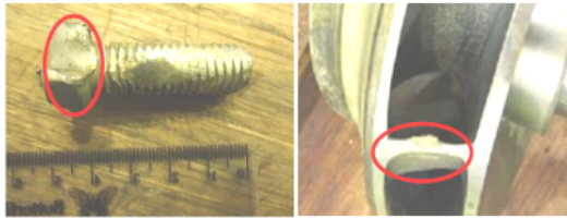
Figure 4. Bolt in pump chamber and damage of impeller
