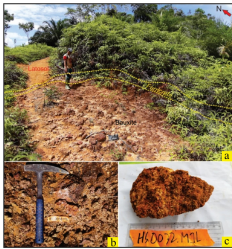
Figure 16. (a) Laterite profile; (b) Outcrop of bauxite zone; and (c) hand specimen of bauxite from granodiorite in the researched area.
