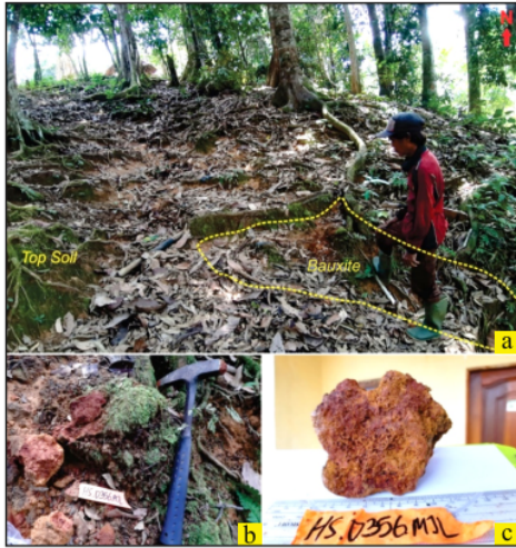
Figure 19. (a) Laterite profile; (b) Outcrop of bauxite zone; and (c) Hand specimen of bauxite from porphyry basalt in the researched area.
