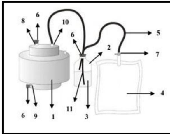
Gambar 1. Digester tipe *continous feeding* (*Continous feeding digester*).
